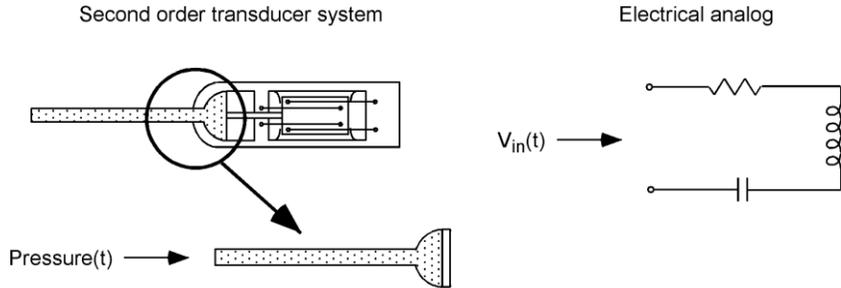
**Figure 2: Simplified physical model of a catheter-transducer system**
