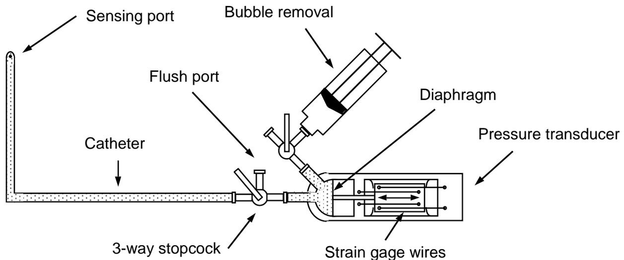
Figure 1: Extravascular blood pressure measuring system
