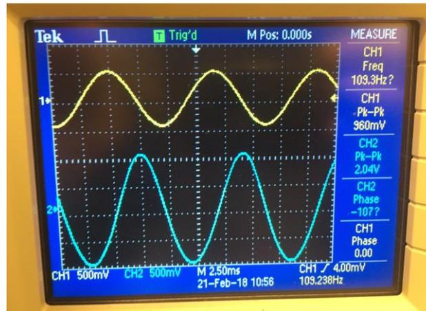
**Figure 5: Sample oscilloscope display for sinusoidal input and output. The measure functions in the right column show values of frequency, Pk-Pk amplitude and Phase, values needed to create a Bode plot.**
