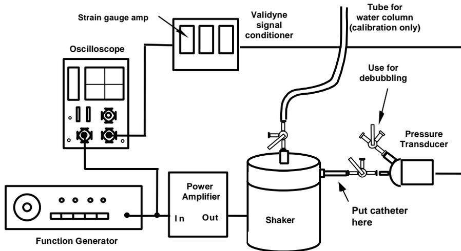
**Figure 4: Schematic of Experimental Set-up. Water column tube is used for calibration only, then removed for the duration of the lab. Stopcocks are shown in an intermediate position that is not normally used during tests.**
