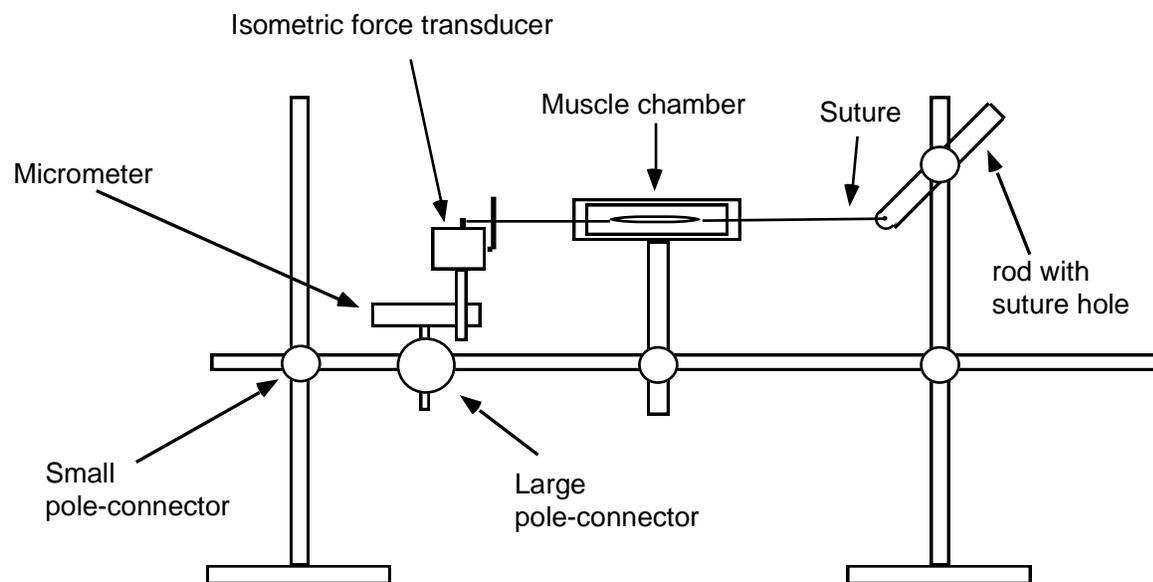
**Figure 1: Experimental setup for isolated skeletal muscle**
