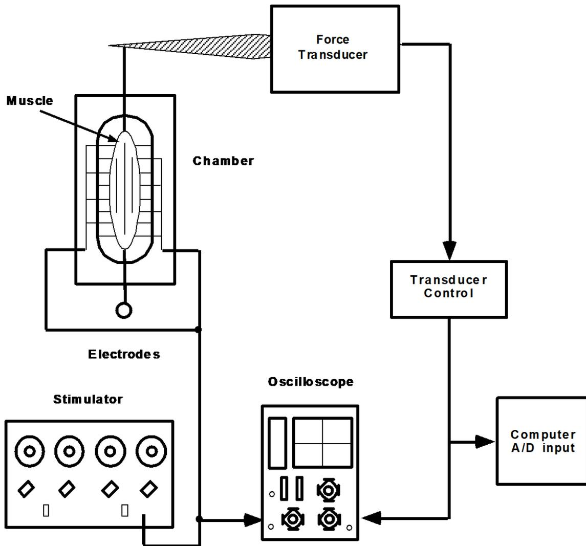
Figure 2: Block diagram for isometric recording
