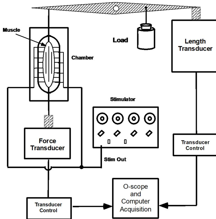
**Figure 2: Block diagram for isotonic recording.**
