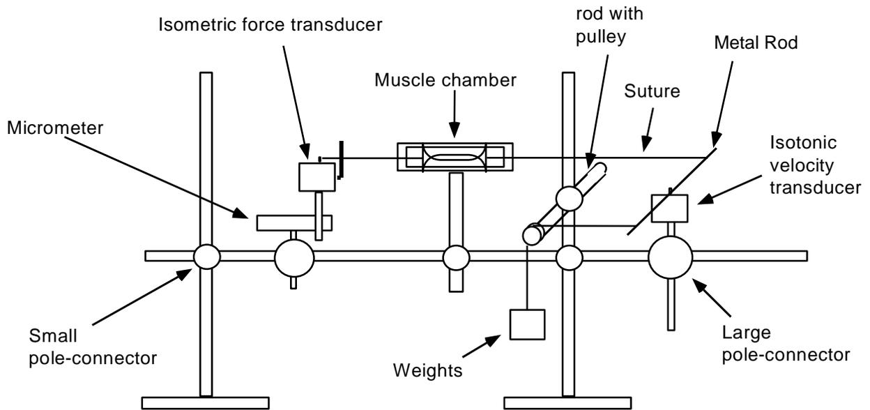
**Figure 1: Force/velocity muscle setup**
