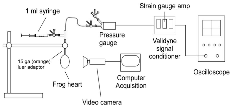
**Figure 2: Experimental setup for the isolated frog heart**
