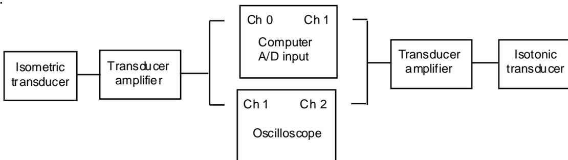
**Figure 3: Wiring Block Diagram**
