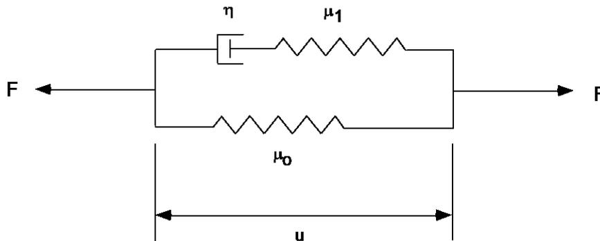
**Figure 1: The standard linear solid model**
