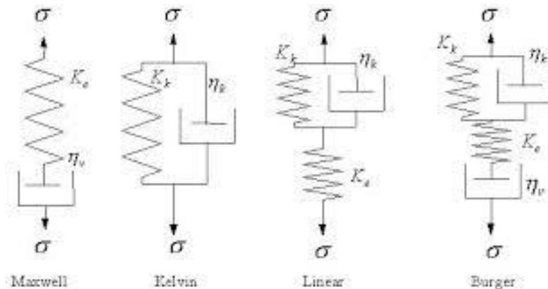
Models with elastic (spring) and viscous (dashpot) elements
