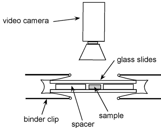
If you can measure the change in distance between the slides (based on the sample thickness and stopper thickness), and then the change in diameter of the sample under load, the Poisson's ratio can be determined. For finite deformations, use the following for Poisson's ratio:
